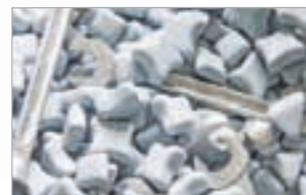
The non-slip, skin-friendly surface is ensured by STAHLWILLE's barrel finishing process.
