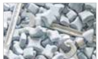
The non-slip, skin-friendly surface is ensured by STAHLWILLE's barrel finishing process.
